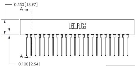
717 Series Ultra-Mate Card Edge Connector - Press Fit
