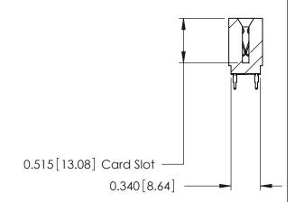
ACAD REFERENCE NO. 746-ENG MASTER 746 Series Ultra-Mate Card Edge Connector - Press Fit DRAWN: J.LEE DATE: AUG 20/09 Part Number: 746-068-560-201 CHECKED: DATE: **EDAC INC** SCALE: SHEET 1 OF 1 THESE DRAWINGS AND SPECIFICATIONS ARE THE PROPERTY OF EDAC INC.,AND TORONTO, ONTARIO SHALL NOT BE REPRODUCED, OR COPIED DRAWING NUMBER CANADA OR USED AS THE BASIS FOR THE 746-ENG MASTER MANUFACTURE OR SALE OF APPARATUS YOUR CONNECTION TO QUALITY & SERVICE WITHOUT WRITTEN PERMISSION.
