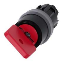
Key-operated switch O.M.R, 22 mm, round, plastic with metal front ring, lock number 73037, red, with 2 keys, 2 switch positions O-I, latching, actuating angle  $90^\circ,\,10:\!30h/13:\!30h,$  key removal O, with laser labeling, upper case and lower case, always upper case at beginning of line
