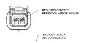
2 POS, RECEPTACLE, PIN, ATM SERIES, SNAP FIT
