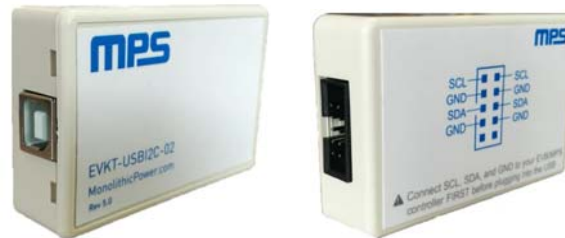
Figure 3: USB to I 2 C Communication Kit
