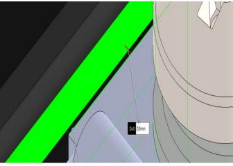
The Link-NP3 and/or Link-NP5 <u>should not</u> be used to parallel connect the 300W dual slot OP A2 or OP A3 modules due to risk of shorting to the module heatsink/configuration chassis. Vox Power will design and release two new parallel links for exclusive use with the 300W OP A2 & A3 modules imminently and will circulate an updated accessory datasheet showing the new links and part numbers.
