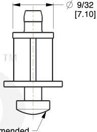
To fit in recommended mtg. hole in 1/16 (1.60) nom. thick board
