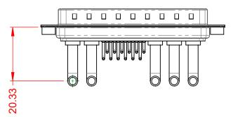
POWER/CO-AX CONTACT RATING: (IF PRESENT) SIGNAL CONTACT CURRENT RATING: 5A PER CONTACT SIGNAL CONTACT RESISTANCE:  $10m\Omega$  MAX. **INSULATOR RESISTANCE:** 5000MΩ min. DIELECTRIC
