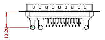
40A (CURRENT) POWER/CO-AX CONTACT RATING: (IF PRESENT) SIGNAL CONTACT CURRENT RATING: 5A PER CONTACT SIGNAL CONTACT RESISTANCE:  $10m\Omega$  MAX. **INSULATOR RESISTANCE:** 5000MΩ min. DIELECTRIC
