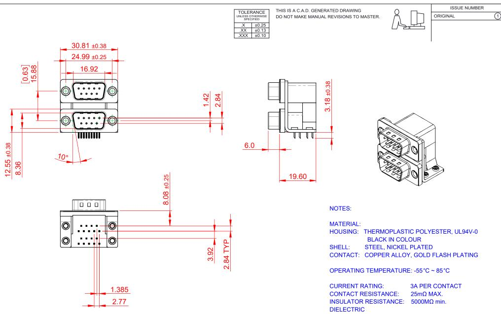
WITHSTANDING VOLTAGE: 1000V AC rms
