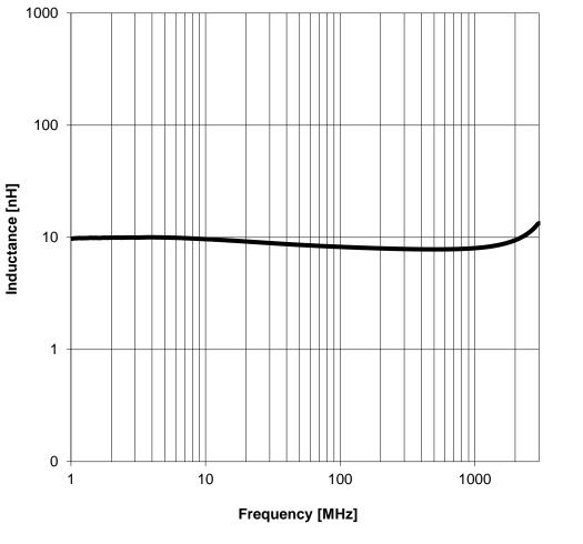
**Typical Inductance vs. Frequency Characteristics:**
