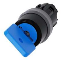
Key-operated switch O.M.R, 22 mm, round, plastic with metal front ring, lock number 73038, blue, with 2 keys, 2 switch positions O<I, momentary contact type, Actuating angle 45°, 10:30h/12h, key removal O, with laser labeling, upper case
