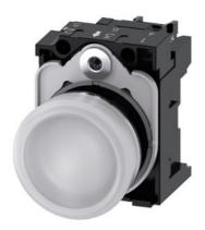
Indicator lights, 22 mm, round, metal, shiny, white, lens, smooth, with holder, LED module with integrated LED 24 V AC/DC, screw terminal, Z=20-unit packaging
