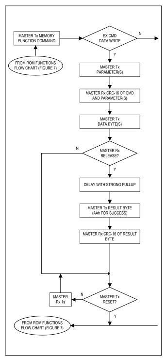
Figure 2. 1-Wire Device Execute Command or Data Write Flow Chart
