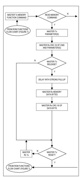
Figure 3. 1-Wire Device Data Read Flow Chart
