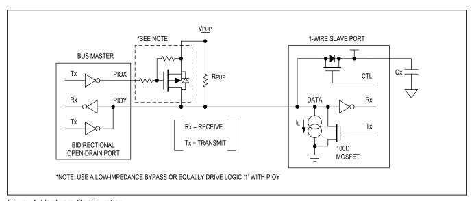
Figure 4. Hardware Configuration
