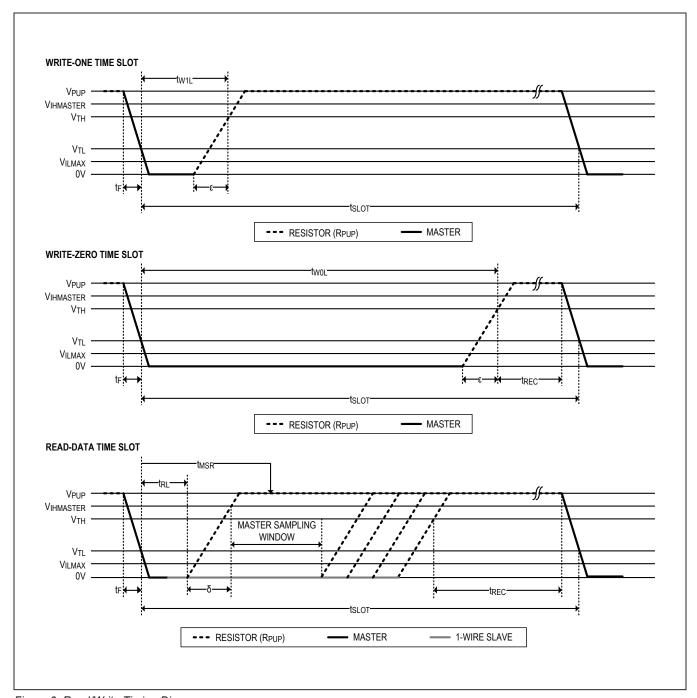
Figure 6. Read/Write Timing Diagrams
