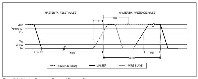
Figure 5. Initialization Procedure: Reset and Presence Pulse
