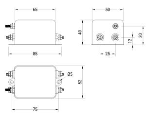
**General Information** Series FLLE2-Q Style **Chassis Mount** Description Single Phase, Chassis Mount Filters Single Phase Features Phase Single-phase RoHS Yes Qualifications IEC/EN 60939, UL, CSA Threaded Studs M4 **Terminal Type**
