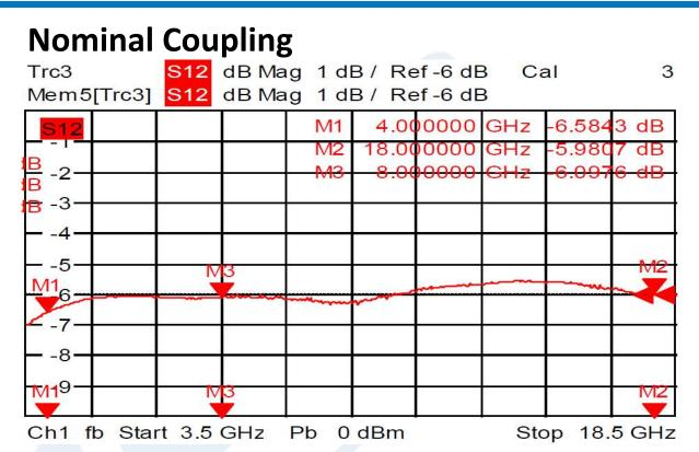
Directional 6 dB SMA Coupler From 4 GHz to 18 GHz Rated to 50 Watts from Pasternack Enterprises has same day shipment for domestic and International orders. Our RF, microwave and millimeter wave products maintain a 99.4% availability and are part of the broadest selection in the industry.
