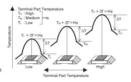
The temperature of the resistor will increase the same △T from the standard terminal part temperature regardlless of the ambient temperature when the same power is applied. This is because there is hardly any heat dissipation from the resistor surface to the ambient air.
