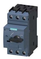
Circuit breaker size S00 for starter combination Rated current 1 A N-release 13 A screw terminal Standard switching capacity
