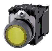
Illuminated pushbutton, 22 mm, round, plastic with metal front ring, yellow, pushbutton, flat, momentary contact type, with holder, 1 NO, LED module with integrated LED 230 V AC, screw terminal
