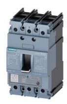
circuit breaker 3VA5 UL frame 125 breaking capacity class H 65kA @ 480 V 3-pole, line protection TM230, FTAM, In=80A overload protection Ir=80A fixed short-circuit protection Ii=5...10 x In cable connection on both sides
