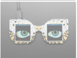
On the left side is a light sensor. It's connected to the seesaw chip on pin 1. Read the analog value using the seesaw library. Lower values like 50 mean its dark. Higher values like 1000 means its bright. It's reverse mount so you can read light levels from the front on the right side of the M4SK.
