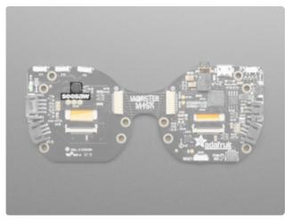
Towards the top center of the left side is the seesaw chip. This chip handles the tactile buttons and the light sensor. You can read the data from them using the I2C seesaw library and the pins specified. This is what lets us have only 9 wires to bridge the two halves of the PCB
