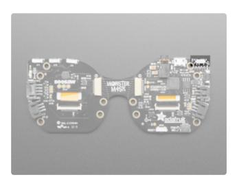
In the upper right corner on the right side is the power switch. You can power off the board when you're not using it to conserve power.
