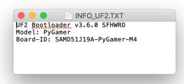
If the bootloader version you see is older than v3.9.0, you need to update. For instance, the bootloader above needs to be upgraded.
