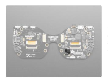
There is an LIS3DH 3-axis accelerometer, on the right side near the bottom towards the middle, connected to the I2C pins for detection motion, tilt or taps.
