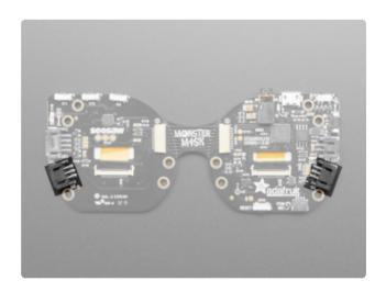
On the right and left sides, towards the bottom, are two connectors labeled D2 and D3. These are 3-pin JST digital or analog connectors for sensors or NeoPixels. These pins can be analog inputs or digital I/O.
