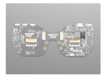
Towards the center left on the right side, next to the microcontroller, is 8 MB QSPI flash for storing graphics and sound effects.
