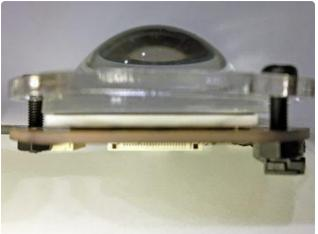
A last-minute change added foam tape to secure the screens. The additional thickness meant that the "12mm-ish" screws won't always make a solid connection. Here's what to do...
