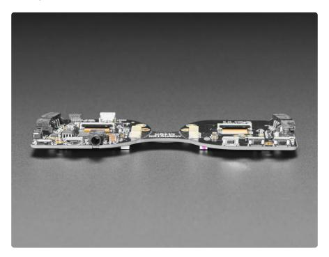
We wanted to make audio-effects easier so in addition to a class D audio amp, there's also a stereo headphone jack that is connected to the two DACs on the chip. Use it when you want an externally sound amplifier box for big effects. For small portable effects, the built-in amp can drive 8 ohm speakers up to 1 Watt.
