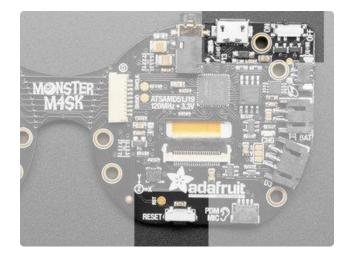
Connect MONSTER M4SK to your computer with a USB cable, set the power switch to the ON position and double-tap the reset button to enter bootloader mode.
