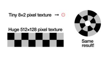
Eye textures can be any size (RAM permitting), on either axis...even down to a single pixel. When wrapping small images around the whole eye, nearest-neighbor sampling (no interpolation) is used. This can be exploited to create stylized blocky or grid designs...no need to waste space on a big image when just a few pixels will do.
