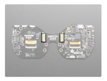
Located on the inside edge of each side is a 9-pin JST SH connector. This connector works with a 9-pin cable and allows you to break the board apart along the perforation, and mount the two halves of the board separately from each other!
