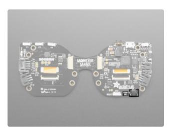
At the bottom on the right side is a 4 pin JST SH port for connecting an optional PDM microphone. Note that the PDM microphone is connected to two SERCOM pins, and we use SPI2 to read PDM data (if you think about it, PDM is just fixed-frequency SPI!) You could in theory turn this into an I2C or UART port. The SAMD51G19 chip used on this board does not support I2S, so we can't use I2S to read the PDM data.
