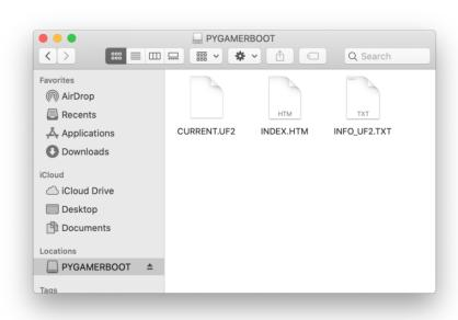
The bootloader version is listed in INFO\_UF2.TXT. In this example, the version is v3.6.
