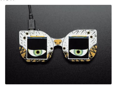
Peep dis! Have you always wanted to have another pair of eyes on the back of your head? Or outfit your costume with big beautiful orbs? The MONSTER M4SK is like the Hallowing () but twice as good, with two gorgeous 240x240 pixel IPS TFT displays, driven by a 120MHZ Cortex M4 processor that can pump out those pixels super fast. You'll get the same quality display as our Raspberry Pi Eyes kit but without needing to tote around a full Linux computer ()
