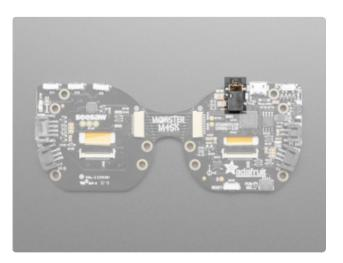
There is a stereo headphone jack on the top of the right side. This is connected to the two analog DAC pins on the SAMD51 - AO and A1
