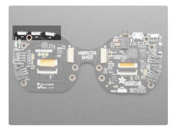
On the left side are three tactile buttons for user interfacing. They are connected to the seesaw chip on pins 9, 10, 11. You need to use the seesaw library to enable the pull-ups on all three and read the buttons (they will be connected to ground when pressed)
