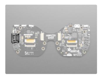
There is a 4-pin JST I2C connector in the center on the left, that is STEMMA and Grove compatible. In CircuitPython, you can use the STEMMA connector with board.SCL and board.SDA, or board.STEMMA\_I2C(). The I2C connection is shared with the seesaw chip and the accelerometer.
