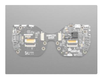
The main processor chip is the ATSAMD51G19 Cortex M4 microcontroller running at 120MHz with 512KB Flash, and 192KB RAM.
