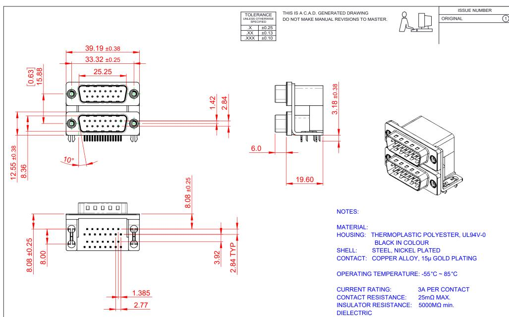
WITHSTANDING VOLTAGE: 1000V AC rms
