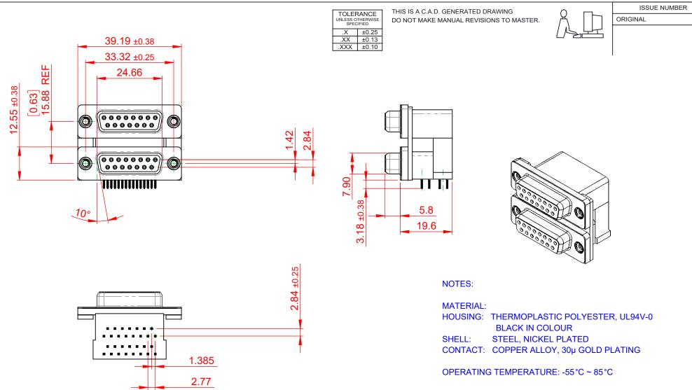
**CURRENT RATING: 3A PER CONTACT** CONTACT RESISTANCE: 25mΩ MAX. INSULATOR RESISTANCE: 5000MΩ min. DIELECTRIC WITHSTANDING VOLTAGE: 1000V AC rms
