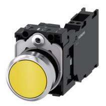
Pushbutton, 22 mm, round, metal, shiny, yellow, pushbutton, flat, momentary contact type, 1 NO+1 NC, spring-type terminal, with laser labeling, inscription or symbol Customer-specific selection with SIRIUS ACT configurator (CIN)
