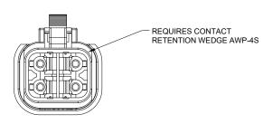
NOTES: UNLESS OTHERWISE SPECIFIED 1. MATERIAL: HOUSING: THERMOPLASTIC SEAL: SILICONE RUBBER
