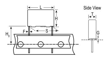
Series F881 Dielectric Metallized Polypropylene Style Radial Features MKP EMI Safety RoHS Lead Wire Leads Safety Class Qualifications ENEC, UL, cUL, CQC AEC-Q200 No THB Performance No Component Weight 4.767 g Miscellaneous ClimCat: 40/110/56/B Shelf Life 104 Weeks
