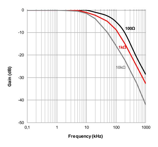
Testcondition:  $I_C = 2mA$ ;  $V_{CE} = 2V$ ; TA = 25°C
