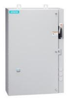
Non-reversing motor starter, Size 1, Three phase full voltage, Solid-state overload relay, OLR amp range 0.25-1A, 208VAC 60Hz coil, Combination type, 30A non-fusible disconnect, Encl NEMA type 4X 304 S-Steel, Water/dust tight noncorrosive, Extra-wide enclosure
