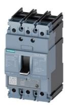
circuit breaker 3VA5 UL frame 125 breaking capacity class S 25kA @ 480 V 3-pole, line protection TM230, FTAM, In=125A overload protection Ir=125A fixed short-circuit protection Ii=5...10 x In cable connection on both sides
