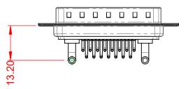
20A (CURRENT) POWER/CO-AX CONTACT RATING: (IF PRESENT) SIGNAL CONTACT CURRENT RATING: 5A PER CONTACT SIGNAL CONTACT RESISTANCE:  $10m\Omega$  MAX. **INSULATOR RESISTANCE:**
