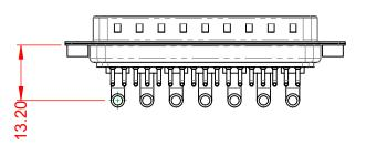
30A (CURRENT) POWER/CO-AX CONTACT RATING: (IF PRESENT) SIGNAL CONTACT CURRENT RATING: 5A PER CONTACT SIGNAL CONTACT RESISTANCE:  $10m\Omega$  MAX. INSULATOR RESISTANCE: 5000MΩ min. DIELECTRIC
