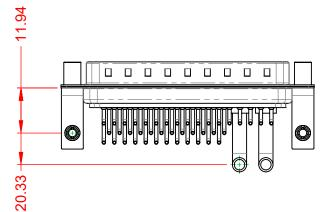
40A (CURRENT) **POWER/CO-AX CONTACT RATING:** (IF PRESENT) SIGNAL CONTACT CURRENT RATING: 5A PER CONTACT SIGNAL CONTACT RESISTANCE:  $10m\Omega$  MAX. **INSULATOR RESISTANCE:** 5000MΩ min.
