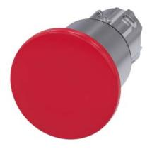
Mushroom pushbutton, 22 mm, round, metal, shiny, red, 40 mm, 3 switch positions, latches after pushing in, unlatches by pull-to-unlatch mechanism to center position, after pulling out the button Retraction to center position, with laser labeling, upper case and lower case, always upper case at beginning of line
