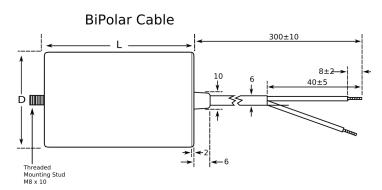
Series C27 Dielectric Film/Foil Polypropylene Style Plastic Case and Cover, Ultra Sonically Welded Description Ultra Sonically Welded Seal, Safety Class PO, **Features** UL 94 V0 Disk RoHS Yes Termination Tin Copper Lead BiPolar Cables UL, VDE, UL (Construction Only), UL\_94 VO Disk Qualifications AEC-Q200 Component 50.77 q Weight
