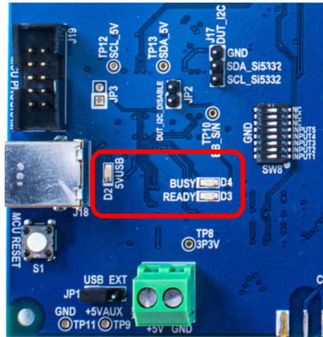
Figure 3.2. Si5332-6A-EVB LED Locations
