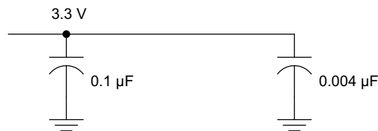
Figure 9-2. Recommended M-LVDS Bypass Capacitor Layout
