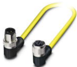
Sensor/actuator cable, 3-position, PVC, yellow, Plug angled M12 SPEEDCON, A-coded, on Socket angled M12 SPEEDCON, A-coded, cable length: 0.5 m
