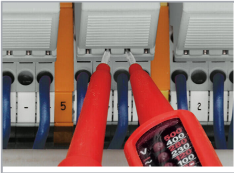
Function testing via touch-proof test slots
