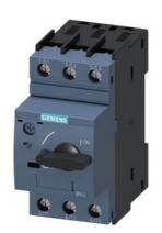
Special type Circuit breaker size S0 for motor protection, CLASS 10 Arelease 13...20 A N-release 260 A screw terminal Standard switching capacity Ambient temperature -50  $^{\circ}\text{C}$  500 switching cycles
