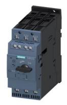
Circuit breaker size S2 for motor protection, CLASS 10 A-release 9.5...14 A N-release 208 A screw terminal increased switching capacity with transverse auxiliary switches 1 NO+1 NC
