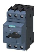
Circuit breaker size S00 for starter combination Rated current 4 A N release 52 A screw terminal Standard switching capacity
