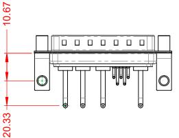
10A (CURRENT) **POWER/CO-AX CONTACT RATING:** (IF PRESENT) SIGNAL CONTACT CURRENT RATING: 5A PER CONTACT SIGNAL CONTACT RESISTANCE:  $10m\Omega$  MAX. **INSULATOR RESISTANCE:**
