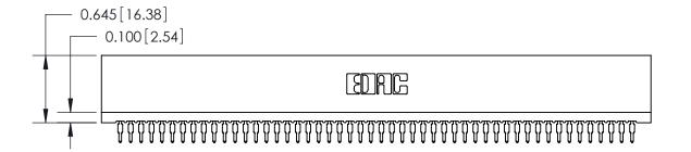
745 Series Ultra-Mate Card Edge Connector - Press Fit
