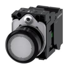
Illuminated pushbutton, 22 mm, round, plastic, clear, pushbutton, flat, momentary contact type, with holder, 1NO, LED module with integrated LED 110 V AC, spring-type terminal, with laser labeling, symbol number according to, ISO 7000 or IEC 60417
