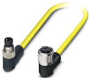
Sensor/actuator cable, 4-position, PVC, yellow, Plug angled M8, on Socket angled M12 SPEEDCON, A-coded, cable length: 1.5 m
