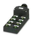
Sensor/actuator box, application: Standard, connection method: M12-SPEEDCON-socket Plastic, number of slots: 8, number of positions: 4, coding: A - standard, slot assignment: single, status display: yes, pnp; master cable connection: Pluggable screw connection 180°, shielding: no
