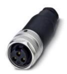
Connector, Universal, 3-position, Socket straight 7/8"-UNF, A-coded, Screw connection, knurl material: Zinc die-cast, nickel-plated, cable gland Pg9, external cable diameter 6 mm ... 8 mm
