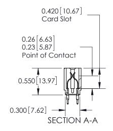
Note: MBB switching contacts assembled in specified positions are available on request. 717 Series Ultra-Mate Card Edge Connector - Press Fit
