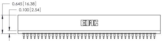
746 Series Ultra-Mate Card Edge Connector - Press Fit Part Number: 746-037-520-506
