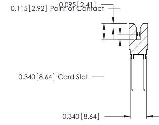
ACAD REFERENCE NO. 746 Series Ultra-Mate Card Edge Connector - Press Fit Part Number: 746-056-541-606 **EDAC INC** THESE DRAWINGS AND SPECIFICATIONS ARE THE PROPERTY OF EDAC INC.,AND TORONTO, ONTARIO SHALL NOT BE REPRODUCED, OR COPIED CANADA OR USED AS THE BASIS FOR THE MANUFACTURE OR SALE OF APPARATUS YOUR CONNECTION TO QUALITY & SERVICE WITHOUT WRITTEN PERMISSION.
